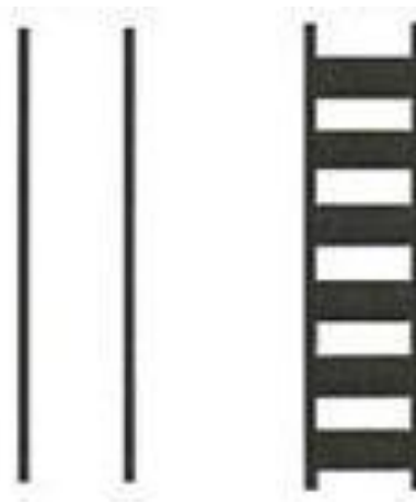
Figure 6 - Crosswalk pavement markings
