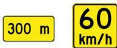
Figure 12 - Curve warning sign tabs
