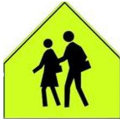
Figure 18 - 'School Area' warning sign
