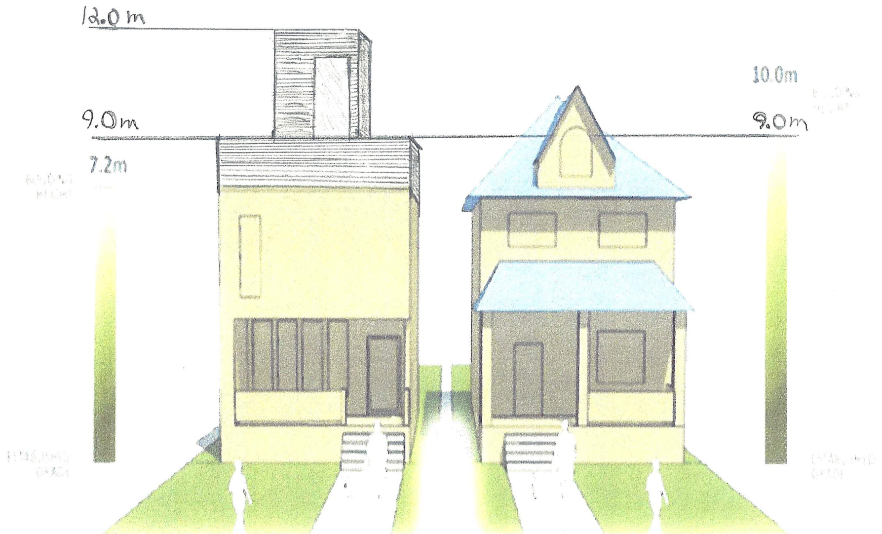
Existing Infill II Proposal: all residential building forms treated alike • Flat roofed house with allowable rooftop projection
